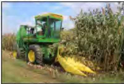
Figure 1. Plots were harvested using a modified John Deere silage chopper equipped with load cells for weighing individual plots.
